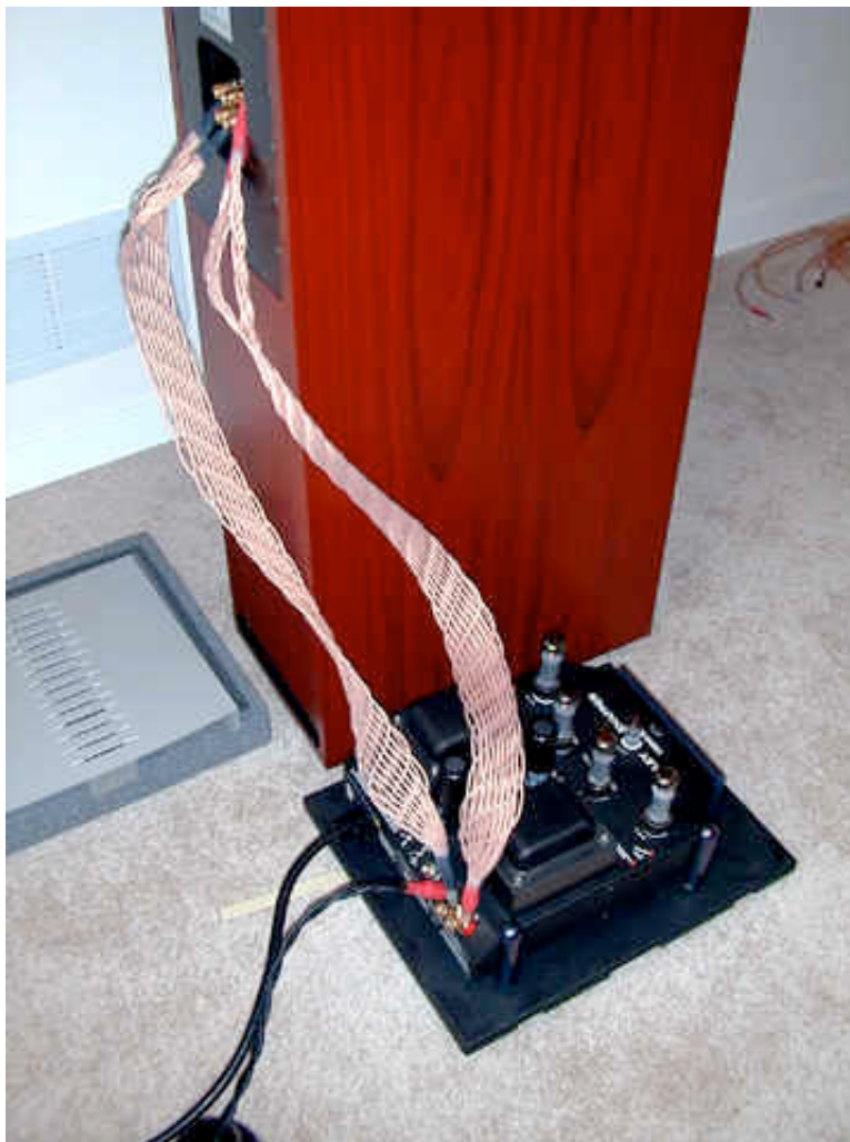
Rear view of the Snapper showing the cabling in balanced mode
