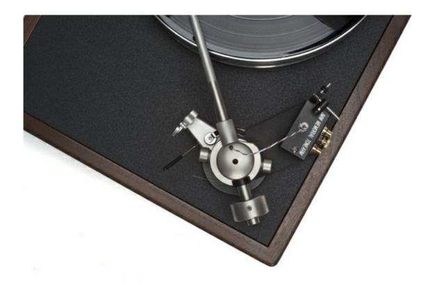
An output pod with RCA jacks and a grounding terminal lurk at the rear corner of the plinth. There's a quick-release connector, meaning tonearm wands are easily interchanged and cartridges effortlessly swapped. And since Lyra's Kleos and Kleos mono cartridges possess identical bodies and parameters, the switch between stereo to mono is a snap.
