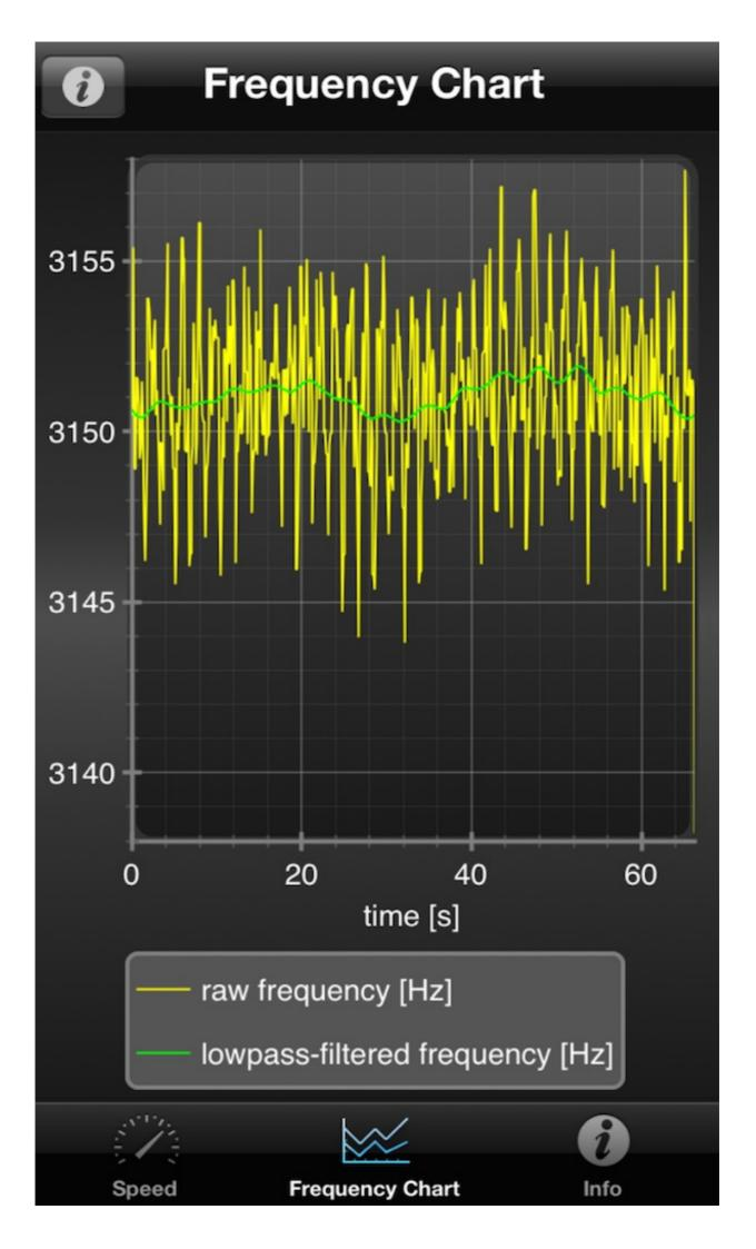
**Chart Info** Done General mean frequency 3151.1 Hz Raw Frequency max deviation (relative) -0.41% / +0.21% max deviation (absolute) -12.8 Hz / +6.6 Hz Lowpass-filtered Frequency max deviation (relative) -0.02% / +0.03% max deviation (absolute) -0.8 Hz / +0.9 Hz
