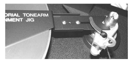
MAKE SURE THE MALE POINT IS IN THE CENTER OF THE FEMALE CUP, IT SHOULD FEEL SOLID BUT YOU SHOULD BE ABLE TO SLIDE IT SIDEWAYS AND THE ARM RAISES AS YOU GO FROM THE CENTER TO THE SIDES OF THE FEMALE BEARING. IT IS AN INVERTED CONE.
