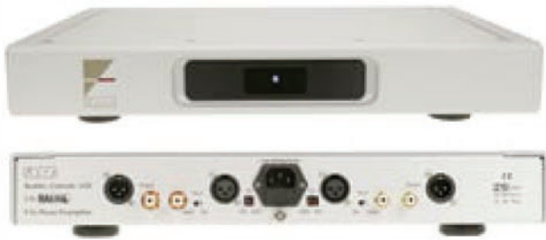
The front is plain bar a logo and power light. The rear features, from left: balanced output, single-ended output, single-ended input, bal/unbal switch, balanced input, and impedance DIP switches (all mirrored on the opposite side). Gain setting is made internally
