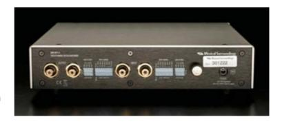
The Grado is rather low level for a MM cartridge but the Nova II allows raising the gain without affecting the 47K loading setting, which some other phono preamps don't allow.
