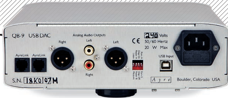
ABOVE: Rather than the usual host of digital inputs, the QB-9 offers USB Type B only alongside single-ended (RCA) and balanced (XLR) analogue outs and AyreLink ports
