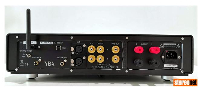
Around the rear of the unit, the ins and outs include one S/PDIF coaxial digital input plus a USB port (24/192KHz). Digital inputs automatically adjust to any of the standard digital audio data rates from 16/44.1KHz to 24/192KHz. To use the USB input with a
