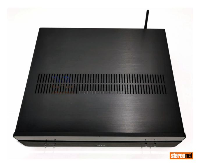
Along the top of the 2 x 105 watts @ 8 Ohms, IA3A integrated amplifier is a row of cutouts in the 4mm-thick aluminium casement for cooling. At first glance, we were not convinced that this would be enough. However, at no point over the time we had the YBA integrated did it ever feel like it was going to overheat.
