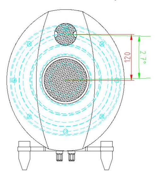
meters, the acoustic centre moves less than 3° degrees, very close to a point source, with evident advantages in terms of soundstage wideness, stability and focalization. An incredible result for an Three-ways loudspeaker.
