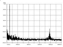
ignore, because it was due to the test setup and would not occur in a hi-fi system), so I have included only the OdB distortion graph, and you can see there's just a 2nd harmonic at –112dB and a 3rd at –109dB and the noise floor is down around –130dB.
