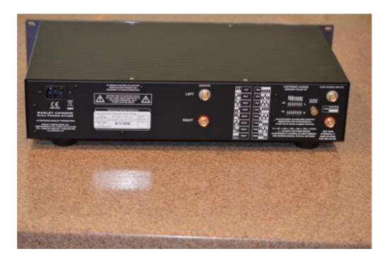
You can set the input capacitance to seven different levels from 50pF up to 350pF. There are 32 different loading possibilities for MC cartridges (which includes the default 47k value) and I used 100 ohms which is how my Krell KPE Reference phono stage is set. The MM input impedance is fixed at 47K ohms. The MM gain is fixed at 45dB and the MC gain is fixed at 60dB. 60dB of gain is more than adequate for the majority of MC cartridges on the market.
